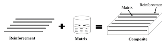
Figure 2 Schematic of FRPs
