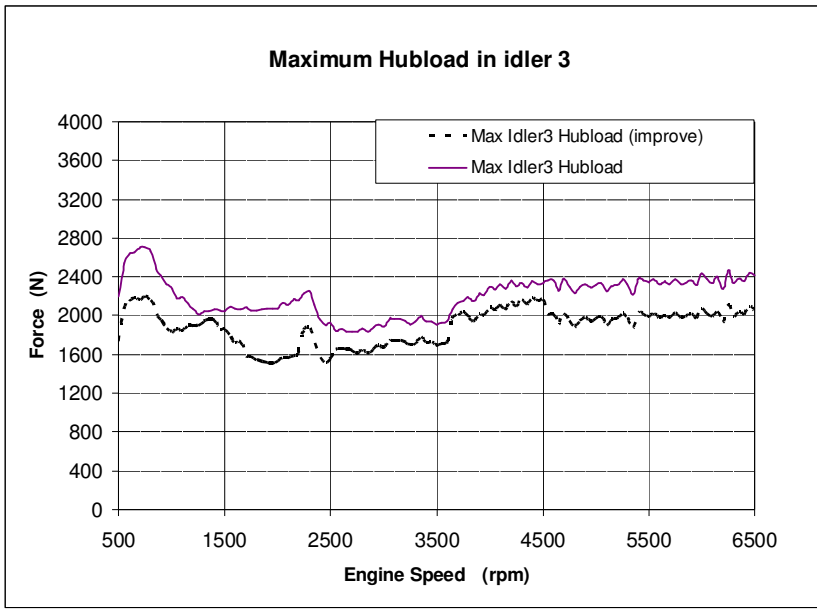
Figure 16. Maximum hubload in idler3( comparison between initial layout and improve layout)
